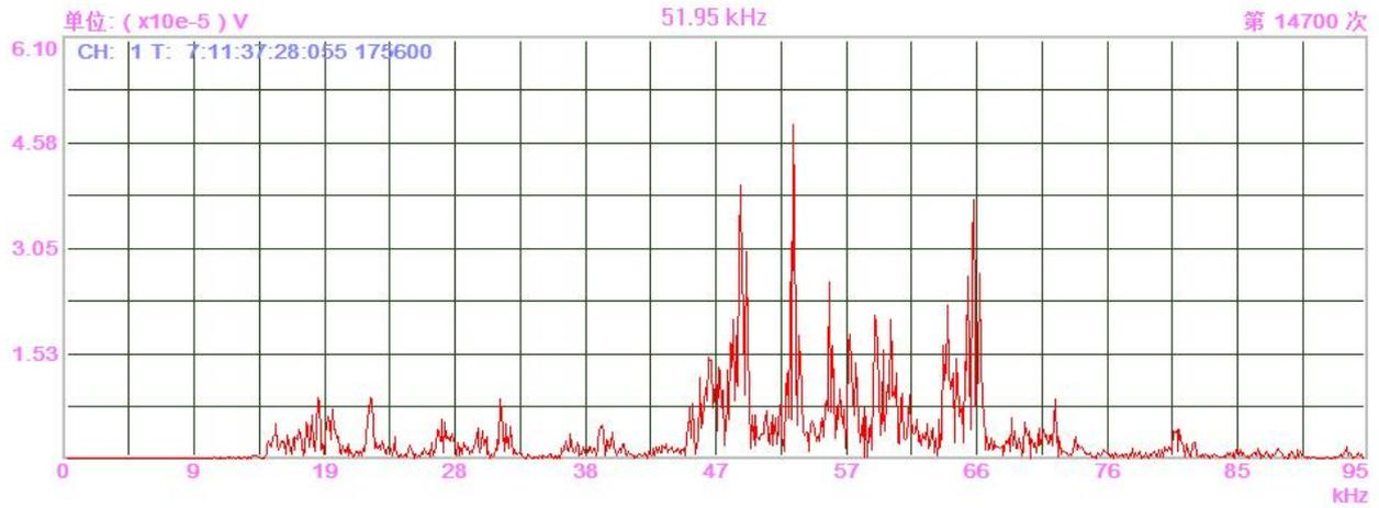
Fig. 5: Typical frequency domain view of leakage
