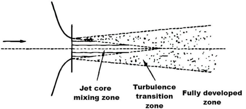
Fig. 1: Pipe jet leakage model
