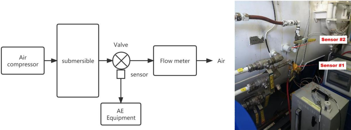
Fig. 2: Experiment connection and the field picture
