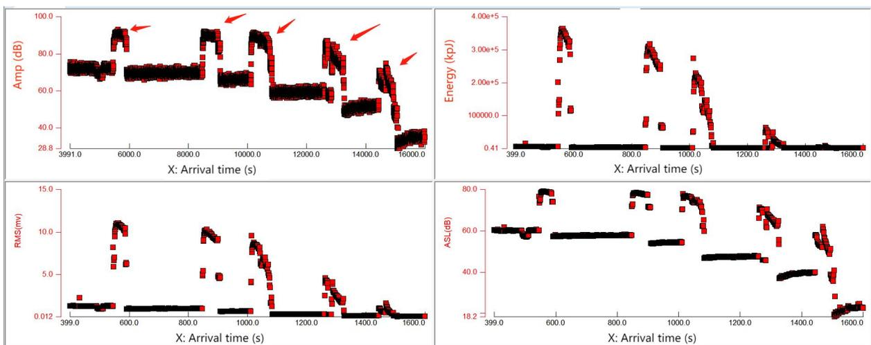
Fig. 7: Continuous waveform in time domain (same valve openings but different pressures)
