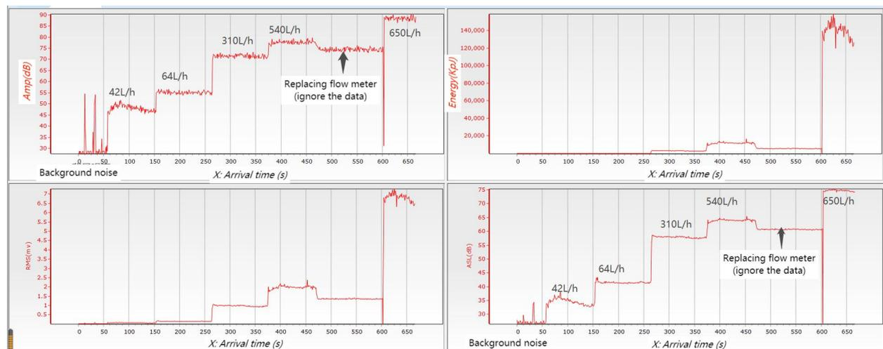
Fig. 4: Different AE feature parameters in time domain under different leakage rates
