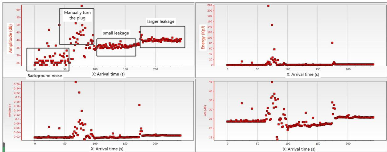
Fig. 11: Plug leakage experiment whole process correlation graphs
