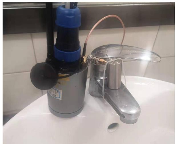
Fig. 12: Online water pipe quantitative leakage experiment system
