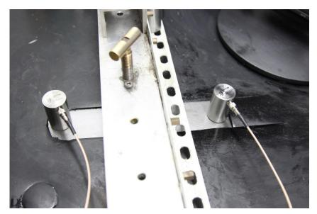
**2.5** Using the spectrum value of the standard sensor given by the Metrology Institute, subtracting the standard sensor's spectrum value of the received signal of this test , thus generate the calibration coefficient of each frequency point of this measurement.
