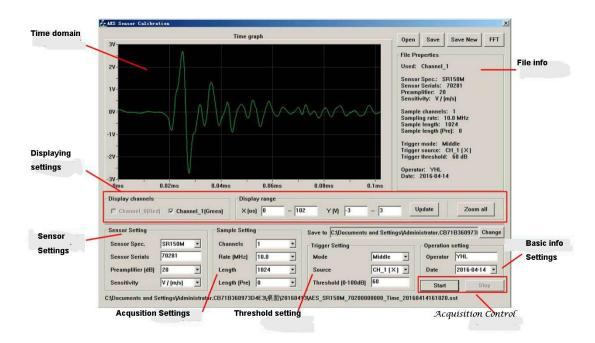
**2.4** The sensor to be calibrated and the standard sensor receive the signal from the same signal source synchronously, and the other channel of the acquisition card receives the signal. The special test software is used for spectrum analysis, which is directly converted to DB value and recorded  $\circ$
