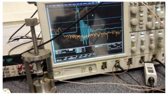
**1.6** The DB value of each frequency point in the frequency domain corresponding to the calibrated sensor shall be archived, the curve shall be drawn, and the standard sensor shall be generated as the secondary calibrated standard sensor
