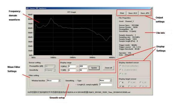
**2.6** Adding the spectrum value which was received by the calibrated sensor of this test to the calibration coefficient described in the pragrahp 1.5 , then obtain the secondary calibration value of each frequency point in the corresponding frequency domain, archive, draw the curve and deliver it to the user for reference.
