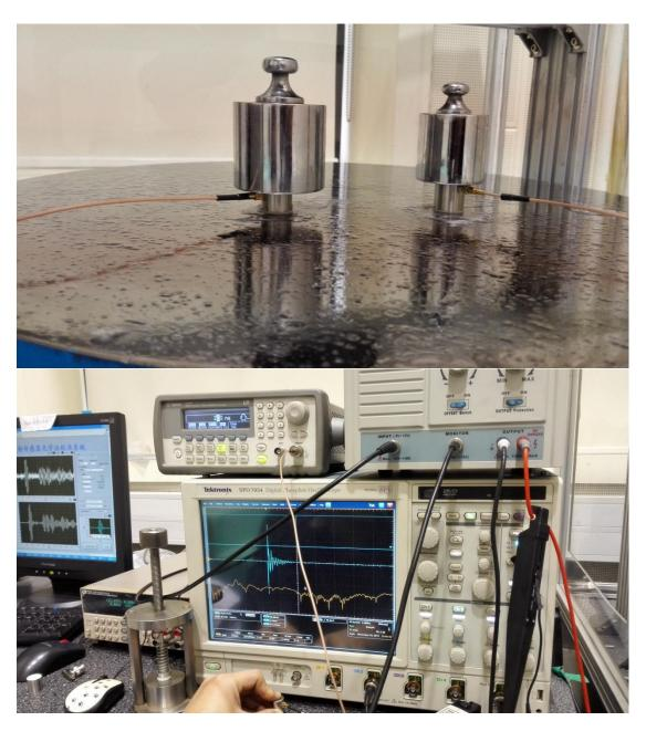
**1.3** The standard receiving equipment adopts the Doppler laser interference vibrometer as the first level standard receiver to receive the vibration signal, with the unit of speed (M / s). The oscilloscope is used for spectrum analysis and recording.
