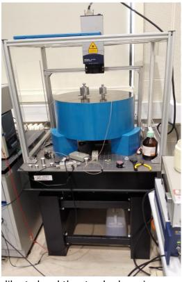
**1.4** The sensor to be calibrated and the standard receiver receive the signal from the same signal source synchronously, and use another channel of the oscilloscope to receive the signal, the unit is voltage (V), do spectrum analysis and record.
