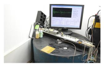
**2.2** On the test bench, use 0.3mm hollow glass tube to send out vibration signal for calibration
