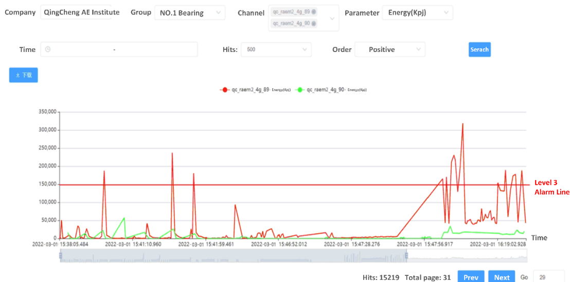
Figure 1: Energy display of qc_raem2_4g_89 channel and qc_raem2_4g_90 channel at 2022-03-01 on NO.1 mechanical equipment.
