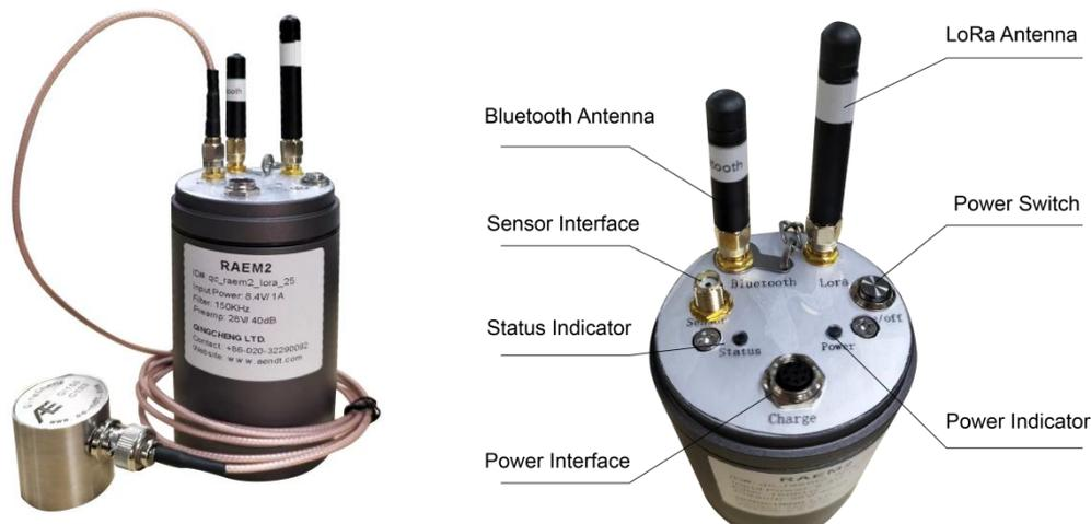
Fig. 2-4 RAEM2 Exterior with External Sensor
