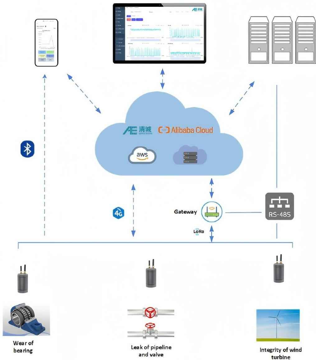
Fig. 1-2 Block diagram of RAEM2 monitoring system
