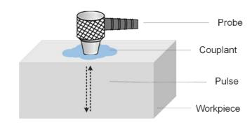
**Note:** To make sure the probe working properly it needs to use couplant to isolate the air between the probe surface and the measured workpiece surface.
